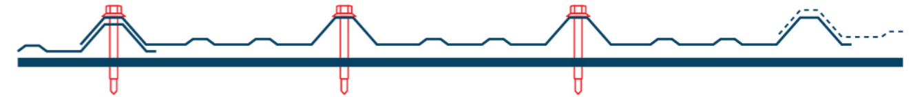
3 FASTENER - END SUPPORT & END LAP
